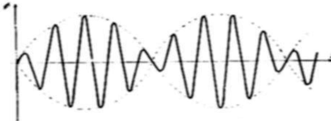
$$\begin{aligned} \phi &= a \sin 2\pi v \left( t - \frac{x}{u} \right) + a \sin 2\pi v' \left( t - \frac{x}{u'} \right) = \\ &= 2a \sin \pi \left[ t(v+v') - x \left( \frac{v}{u} + \frac{v'}{u'} \right) \right] \cos \pi \left[ t(v-v') - x \left( \frac{v}{u} - \frac{v'}{u'} \right) \right] \end{aligned}$$
